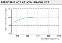
Typical module performance under low irradiance conditions in comparison to STC conditions (25  $^{\circ}\text{C},$  1000 W/m²).
